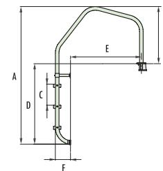
EN Made of Ø43 AISI-304 stainless steel handrails (AISI-316 available on order).
